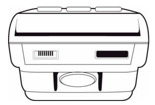
Figure 3 The V<sup>x</sup>670 Primary Port (Bottom View)
